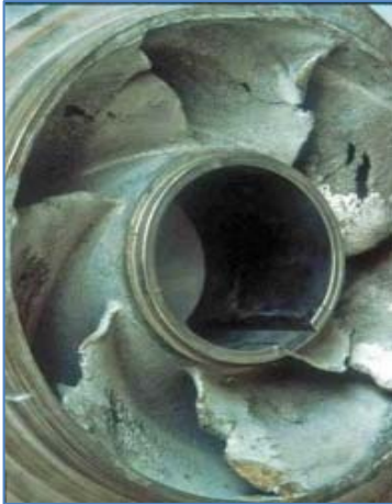
Figure 3: Example of cavitation damage in a pump impeller (Source: www.waterworld.com )
